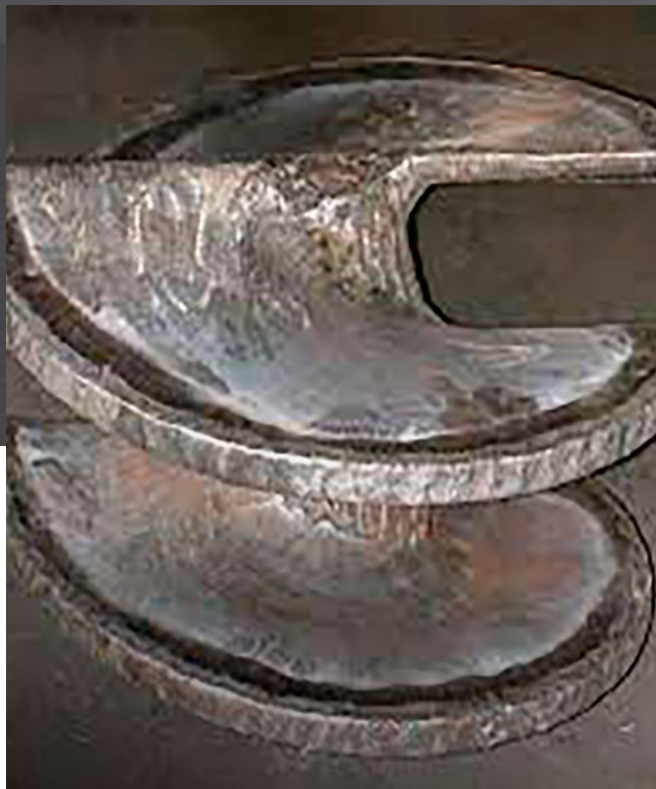
Extruder propeller with anti-wear coating
