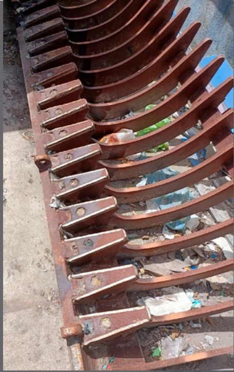
Shredder spare parts - Before and after regeneration
