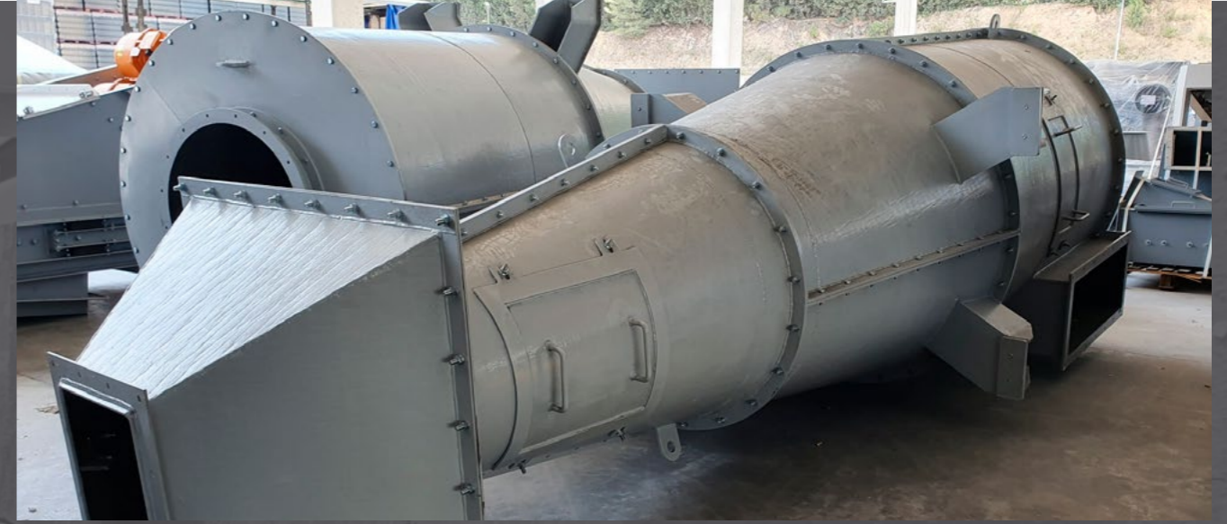
Cyclone with dispenser for glass recycling plant
