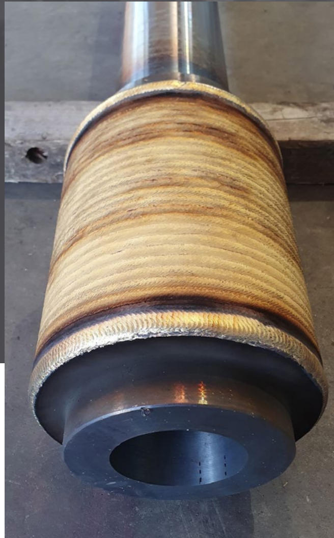
Bushing reconstruction in CuAl8
