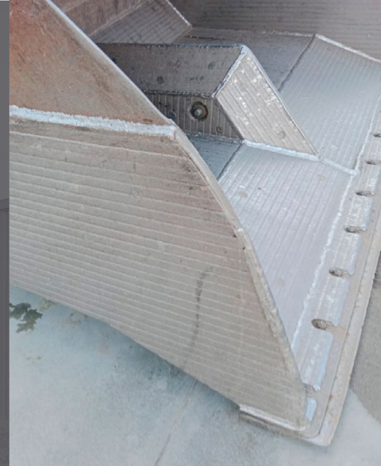
Bucket covered with clad wear plate
