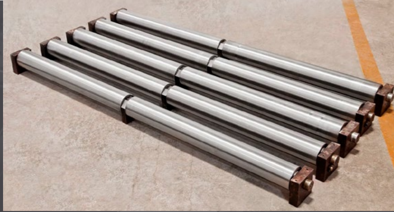
Continuous casting rollers and liners
