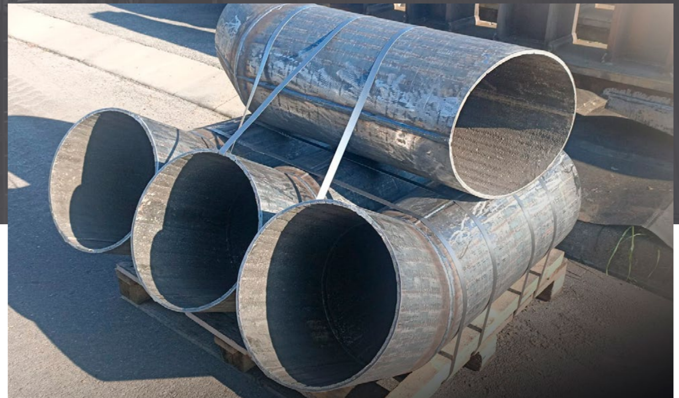
Pipes made of cladded wear plate
