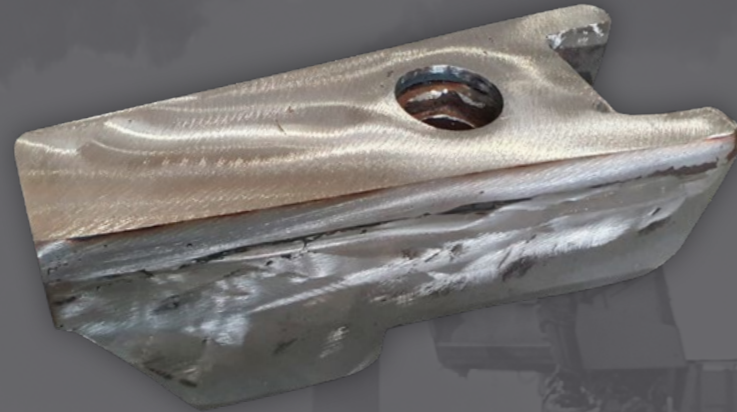
Shredder spare parts - Before and after regeneration
