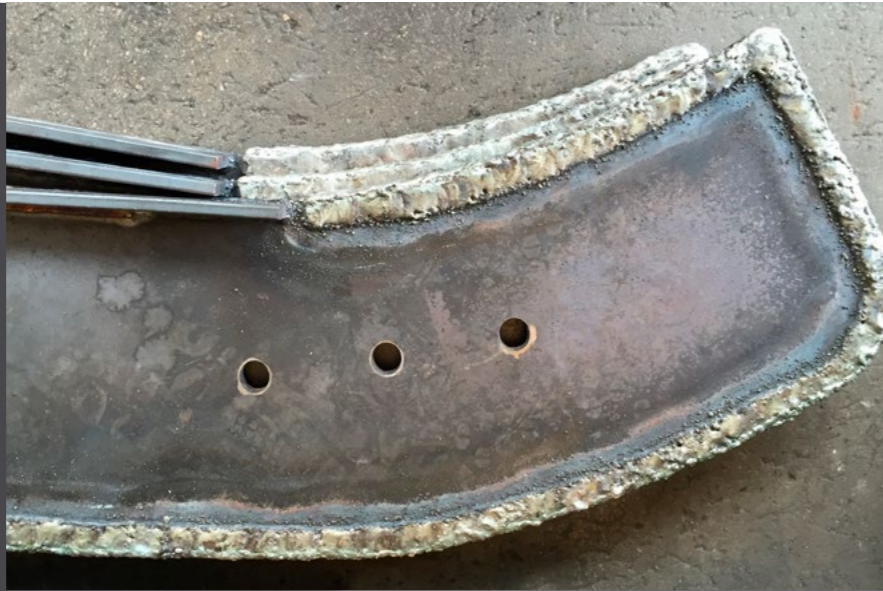
Shovels for foundry with tungsten carbide coating
