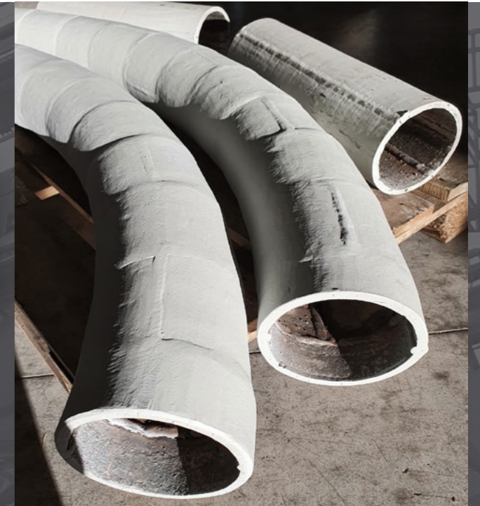
Pneumatic conveying tubes
