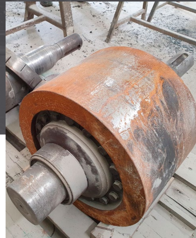
Ceramic aggregates grinding cylinder - Before and after regeneration
