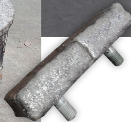
Impeller hammer with anti-wear coating
