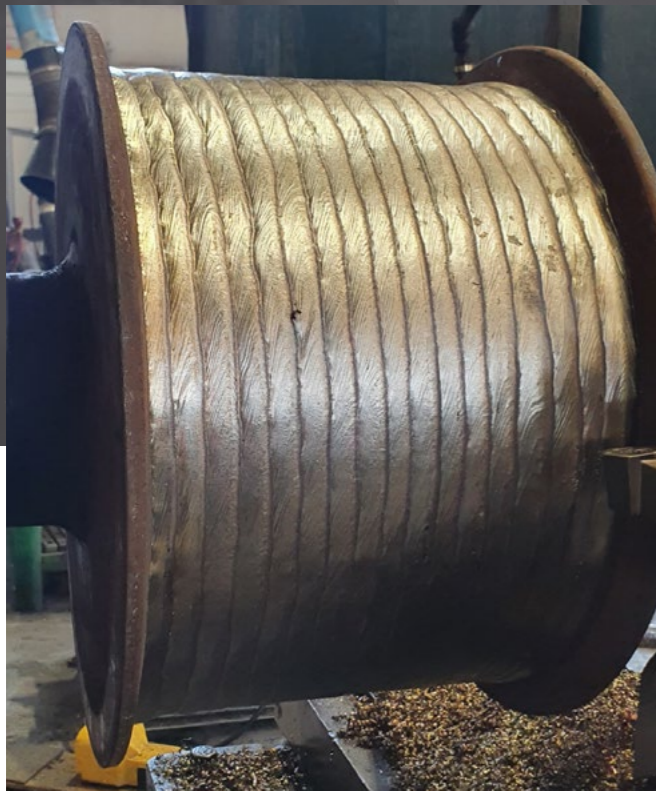
Billet rollers - Before and after regeneration
