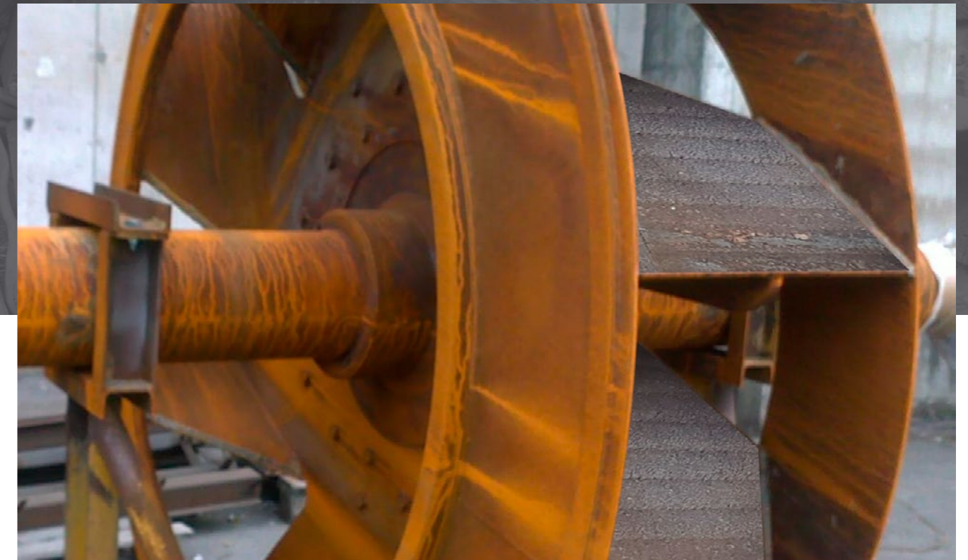
Impeller and nuts with wear protection
