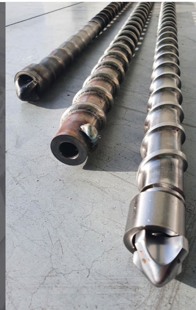
Extruder screws Before and after regeneration
