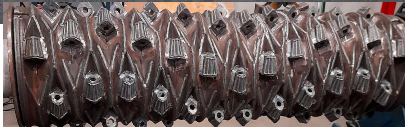
Waste shredder - Before and after regeneration
