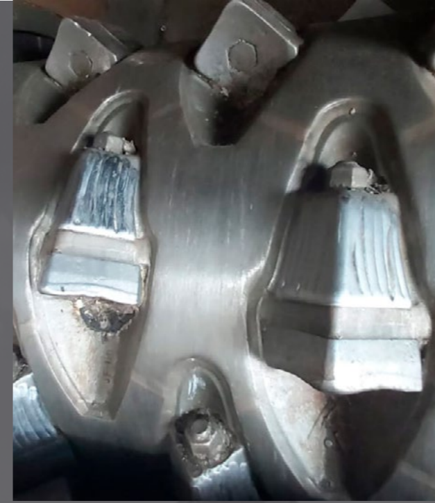
Waste shredder - Before and after regeneration
